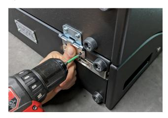
Level the hinge (just above the slide bolt on X Series boards) and tighten the first screw to hold the hinge in position. Do not over tighten.
