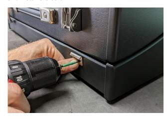
Level the clip and then tighten the screw, being careful not to over tighten it.
