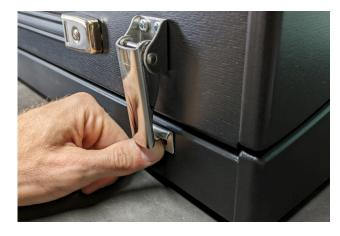
Pre-drill the first hole a 1/4" deep with an 1/8" bit and install the screw.
